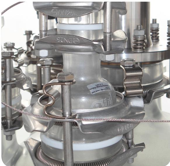
Fig. 4: Potential equalization connection
