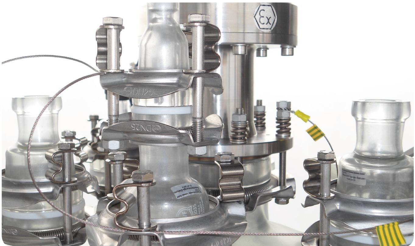
Fig. 1: Potential equalization of metal flanges by means of attached stainless steel cables
